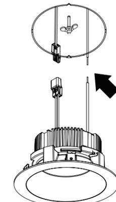
**9** Connect module female connector to hardwire adapter male connector.
