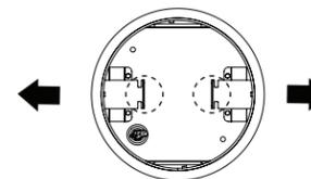
**6** Connect hardwire adapter (included) to junction box electrical leads.
