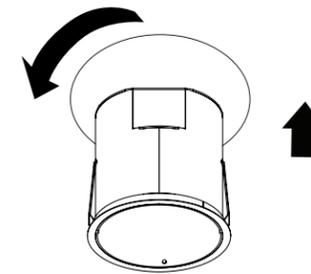
**5** Push the push flanges on the spring clips out, making sure that the notches on the spring clip fully interact with the T-shaped cutout in the housing.
