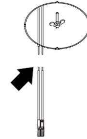
**7** Align trim onto module and turn trim clockwise until secure.
