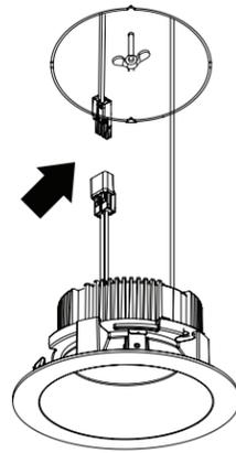
**10** Place module into junction box. Push trim up until flush with ceiling.
