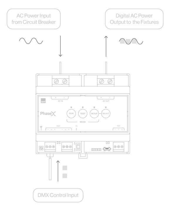
The PhaseX Gateway is the heart of any PhaseX installation, and provides filtered AC Output with DMX data to fixtures.
